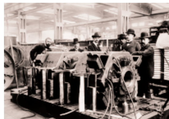
Test stand for locomotive engines, 1895. In the centre of the picture is Charles Brown.
