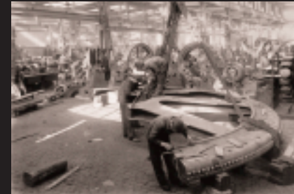
Generator assembly in Baden, 1895
